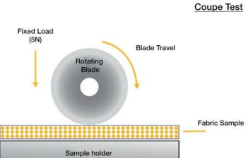
The coupe test has proven to be unreliable for high cut resistant materials due to blunting of the blade during the test to produce inaccurate results.
